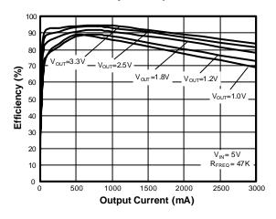
Efficiency vs. Output Current
