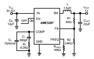
Figure 2. 1V at 3A Step-Down Regulators.
