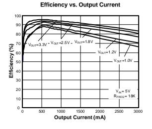
Efficiency vs. Output Current
