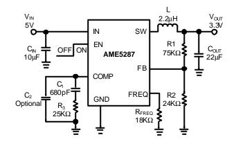
Figure 1. 3.3V at 3A Step-Down Regulators.
