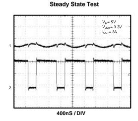
1)  $V_{OUT}$ = 10mV/div 2)  $V_{SW}$ = 2V/div
