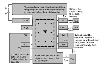
Figure 3. AME5287 Regulators Layout Diagram
